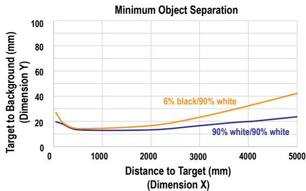
Figure 25. Minimum Object Separation for 50 ms Response Time
